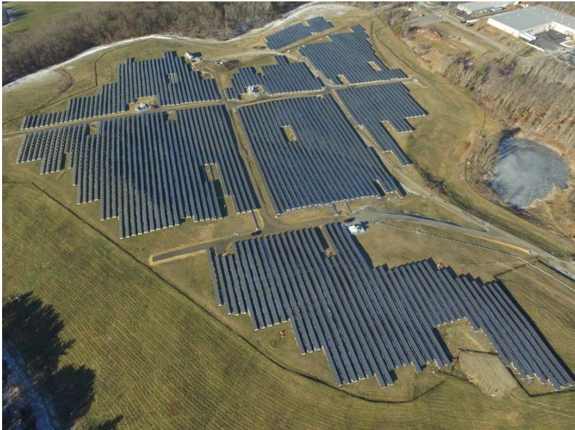
Location: Amesbury, MA Size: 6.0 MW Technology: Ballast on landfill
